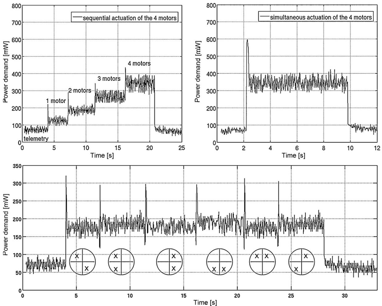
Fig. 6. Measurement of power absorbed by the control/locomotion module related to sequential (top-left) and simultaneous (top-right) actuation of the 4 motors. At the bottom, a 3D locomotion strategy based on the simultaneous use of only two motors.
