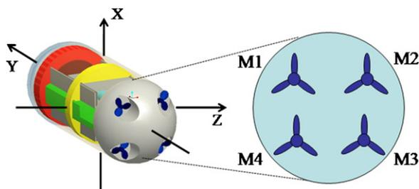
Fig. 3. Schematic of the locomotion system and actuation diagram of the propellers.
