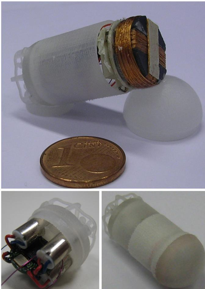
**Fig. 4.** Integration of the power module and the locomotion module in a single capsule. The details depict a magnified view of the ZigBee  $\mu$ C and motors (bottom-left) and the assembled capsule (bottom-right).
