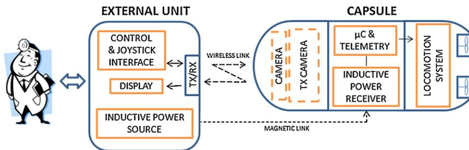
Fig. 1. Block diagram of the wireless power, self propelled and steerable capsule.
