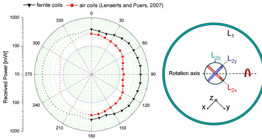
Fig. 5. Compared measurements of the power received by ferrite- and air-coils (Lenaerts and Puers, 2007) for an external mmf of 65 ampere-turns. The dotted lines represent an extrapolation of the measurements to the full 360°. Note: The power scale is logarithmic. The relative position of primary, secondary coils and the rotation axis are resumed in the scheme at the right.
