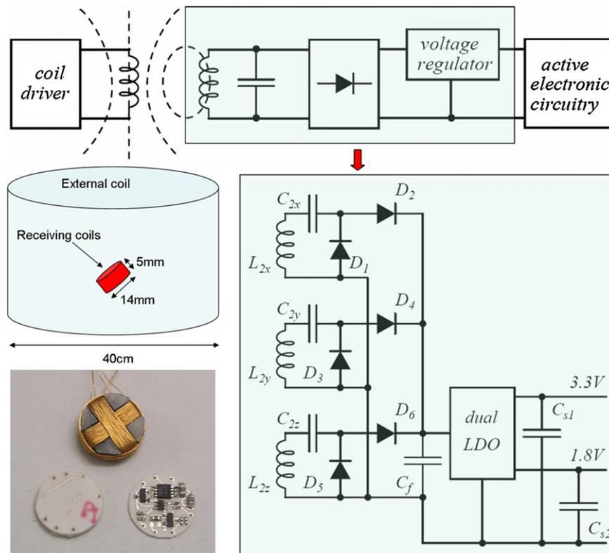
**Fig. 2.** General principle underlying inductive powering systems (top) and schematic of the multiple receiving coil-set (right). At the left, spatial arrangement of the coil composing the power module (top) and a detail of the 14 mm ferrite-coil receiver before assembling (bottom).
