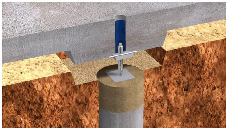
Figure 3: Tella Firma Pier and Slab System<sup>11</sup>
