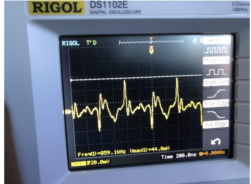
Waveform of the photodiode voltage output
