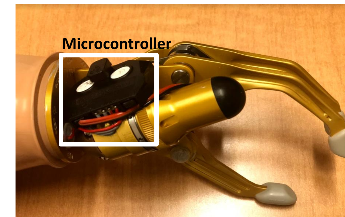
Figure 12: Image of Ottobock myoelectric prosthetic hand with integration points highlighted
