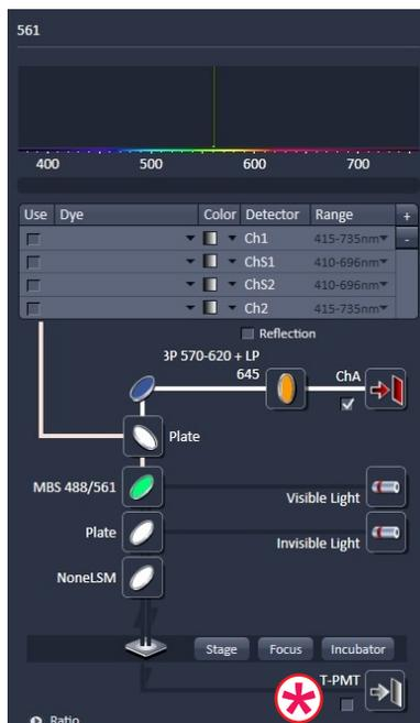
5. The Airyscan light path (shown above) is significantly different from the normal confocal path, i.e. there is no control over the emission bandwidth and no DIC image is possible, **DO NOT CHECK THE T-PMT BOX, \*** DOING SO WILL REQUIRE YOU TO RELOAD YOUR CONFIGURATION.
