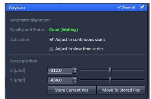
11. If one or more colors cannot be optimized enough to get the best Quality and Status setting, try manually changing the “Servo Position” in X and Y **1**. When the Honeycomb looks as close to ideal as possible, turn on all channels and click “Snap” for a single 2D image.
