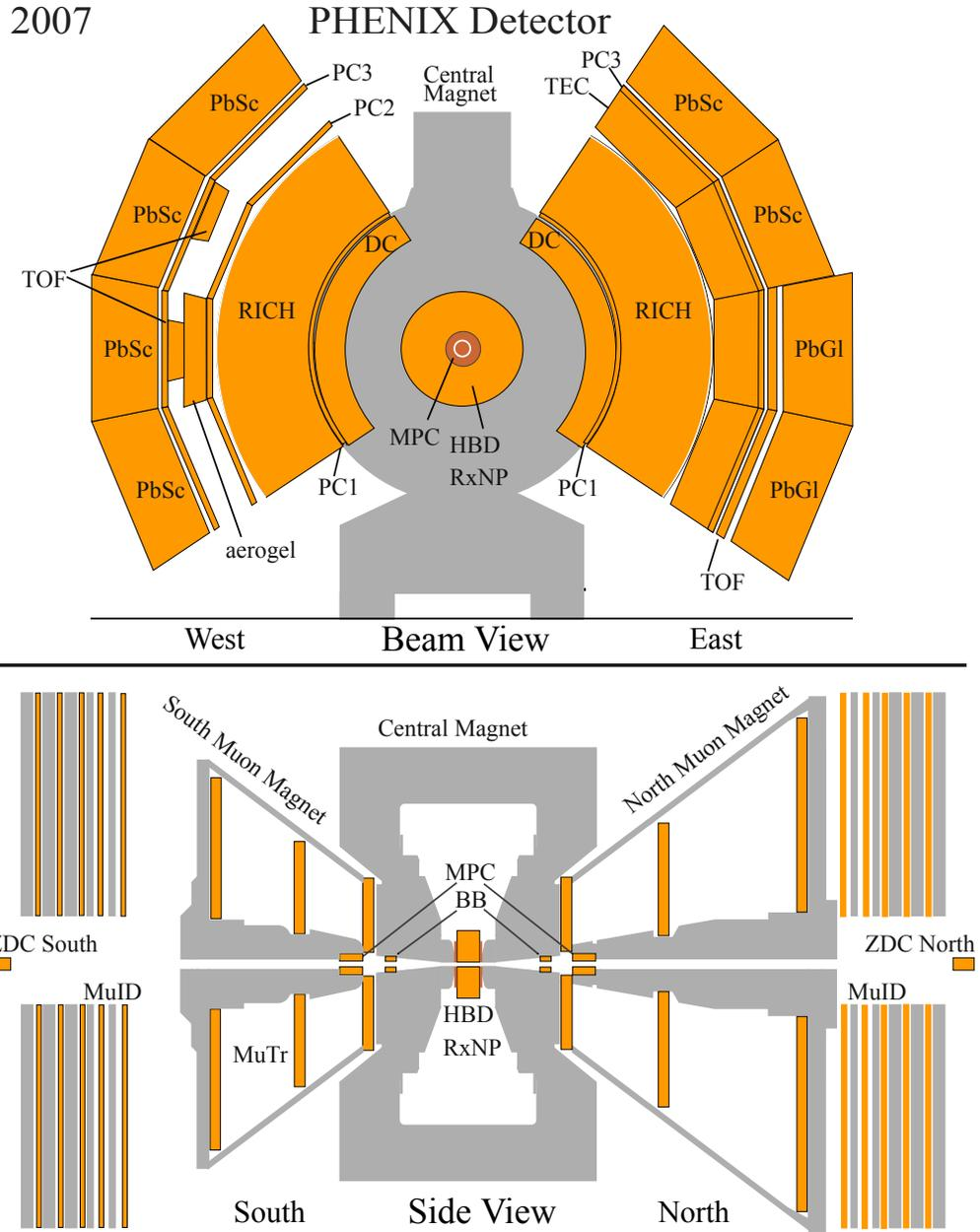
**Figure 2.4:** Schematic of the PHENIX experiment setup in the 2007  $Au + Au$  run (Run7). Top: Cross section of central arms perpendicular to the beam pipe. Bottom: View from the side with the beam pipe spanning the horizontal direction.
