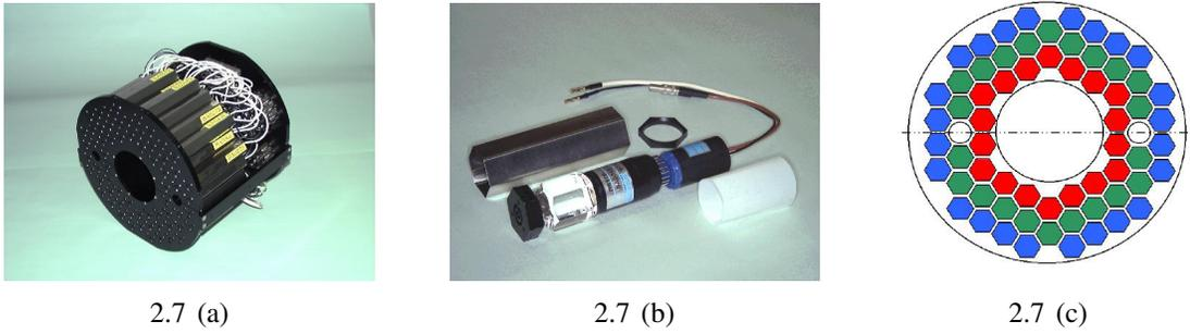
**Figure 2.7:** (a) Picture of the 64 PMTs comprising the BBC array. (b) BBC element consisting of one inch mesh dynode PMT mounted on a 3 cm quartz radiator. (c) Schematic of the BBC, with each box corresponding to a PMT.
