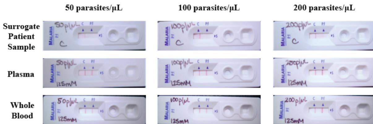
**Figure 7.** Improvement in the visual limit of detection of the SD BIOLINE malaria RDT after extraction from either plasma (middle) or whole blood (bottom) for 50 (left), 100 (middle), and 200 (right) parasites/ $\mu\text{L}$  as compared to mimic patient samples (top). The elution chamber from an extracted sample was spotted on the RDT and developed according to the manufacturer's specifications.
