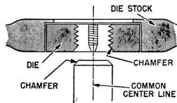
The chamfer helps the die engage the round stock to start the external thread cutting
