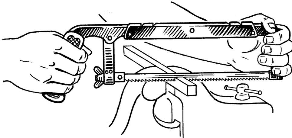
Hacksaw (note the blade teeth orientation and the proximity of the cut to the vise)
