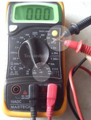
Multimeter in continuity mode with probes touching
