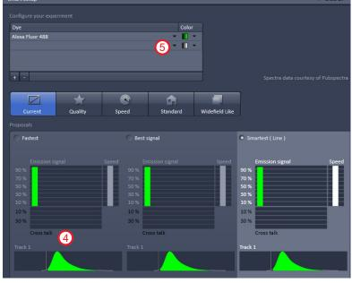
**12**. After the configuration is loaded, the menus within the setup manager are updated to show which track has which color(s) in "imaging setup" (1) as well as the pre-configured light path for each track (2). The highlighted (blue bar) track is the one shown in the light path (3). In the example shown here, "smartest" configuration was chosen in smart setup so there are two tracks with two colors in each track.
