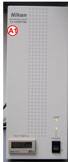
The Hg lamp should not be cycled quickly; let it equilibrate for at least 15 minutes before turning it off again, and let it cool for at least 15 minutes before turning on again. It is essential for the Hg lamp to COOL DOWN before it is fired again or it may be damaged.
