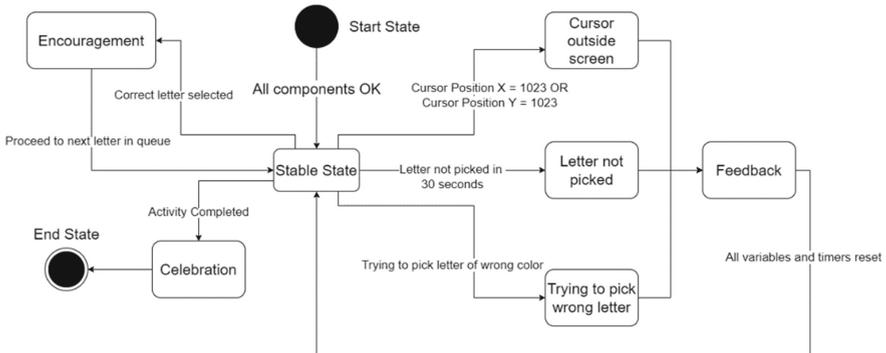
Fig. 7. State machine for the main levels
