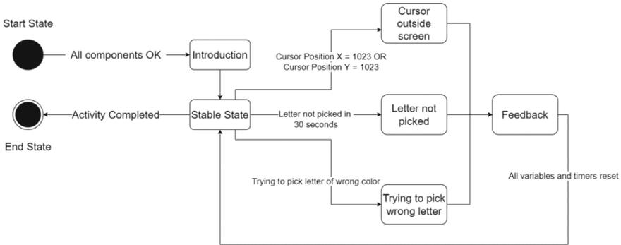
Fig. 6. State machine for the tutorial level
