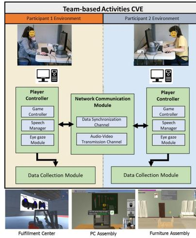
Fig. 1. System setup and snapshots of all three collaborative tasks
