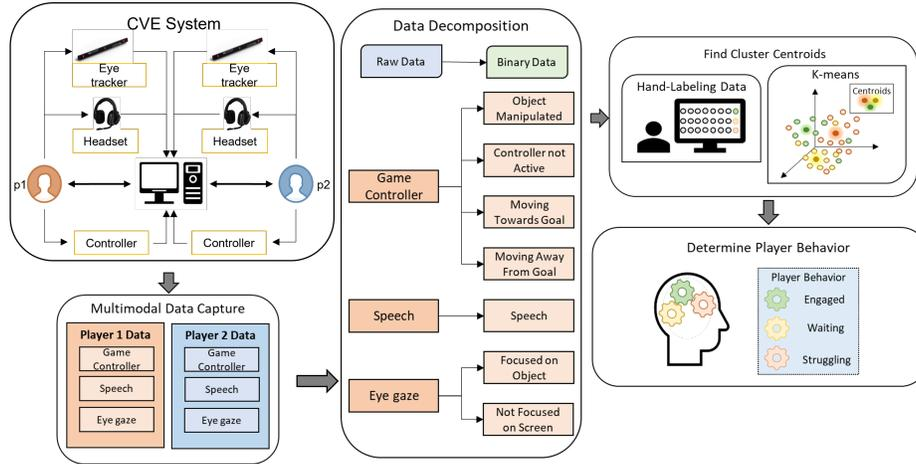
**Fig. 2.** Workflow for automated labeling
