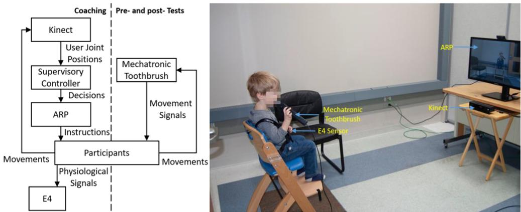
Fig. 1. System architecture and setup.
