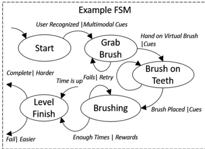
Fig. 6. An example FSM showing different states of the medium difficulty level.
