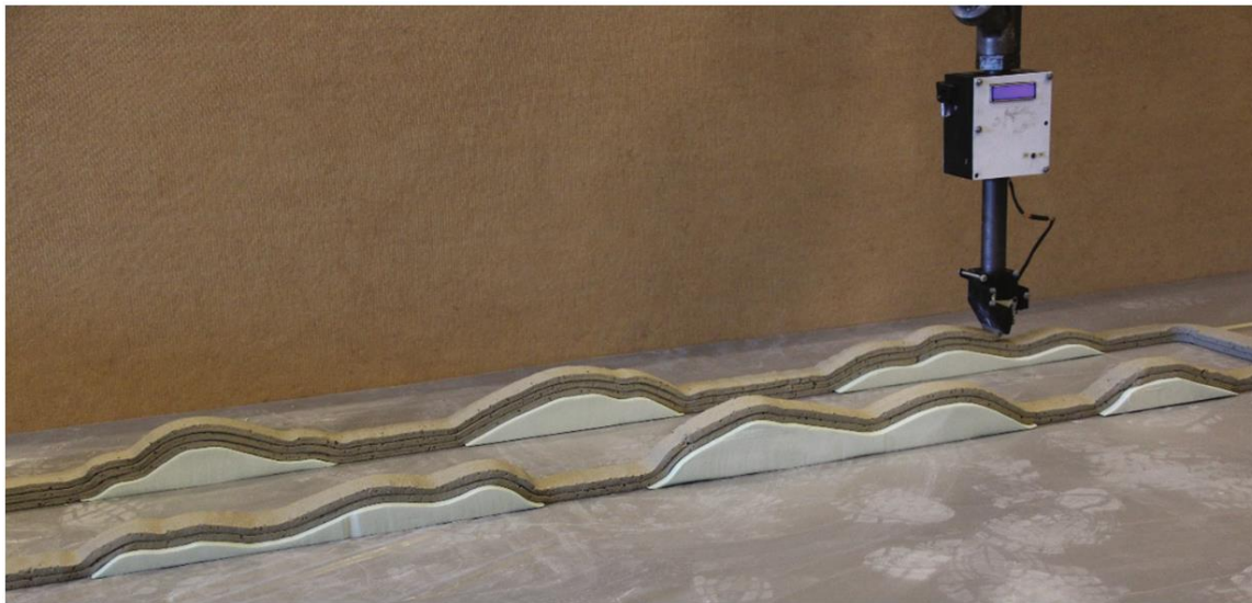
Figure 8 - 3D printing concrete on a non-flat surface with arbitrary curvature and height variations. Adapted from [19].
